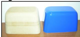
tapered sides for the mould
